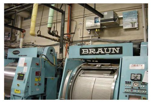
Figure 3. EcoTex<sup>TM</sup> ozonation equipment (wall-mounted) above two Braun Washers.
